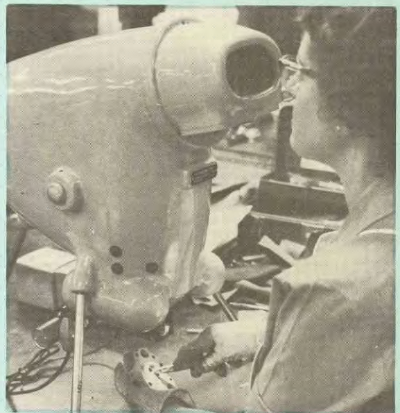
Binocular microscope used to deburr precision pump parts.
