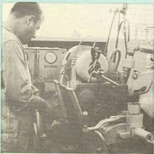
Grinding gear set journals on a Cincinnati angular head grinder.
